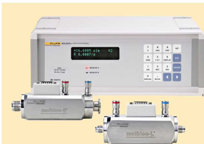
The molbox1 + flow terminal displays the results of flow measurements from either the molbloc-L laminar flow element or the molbloc-S sonic flow nozzle, and provides on-board leak detection.
