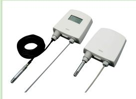
A market leader in humidity sensors & transmitters, Vaisala's HMT120 Humidity Transmitter offers accurate humidity measurements of both rooms and storage Chambers over the full range of 0-100% RH. Accuracy of 1.5%RH with stability as good as 0.5%RH per annual calibration cycle ensures measurement peace of mind.
