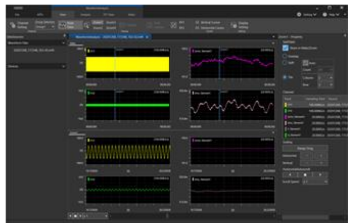
Synchronous display of DL950 waveform data and WT5000 power data
